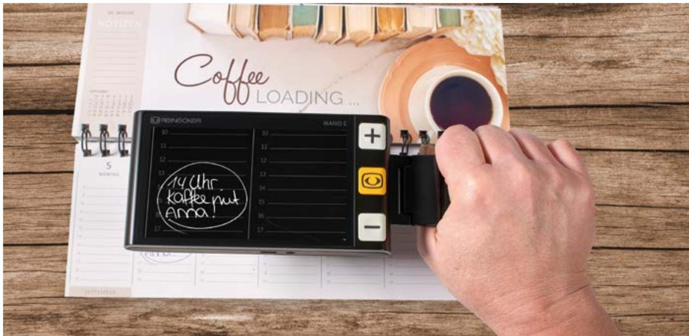
MANO 5 has a low-reflection, matte display and magnifies the reading material continuously up to 20x. The folding handle enables use like that of a conventional hand magnifier. With the stand folded out, you can also write under the magnifier without having to hold it in your hand at the same time.
